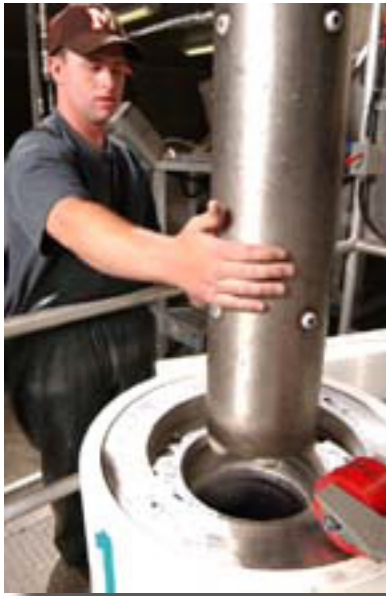
David Morrison, at the Nisbet oyster processing plant near Willapa Bay, maneuvers a stainless steel canister full of raw oysters and water into a high-pressure chamber. The oysters will be exposed to 45,000 pounds per square inch (psi) of pressure, killing bacteria and automatically shucking the oysters in the shell. Photo: Lynn Ketchum
