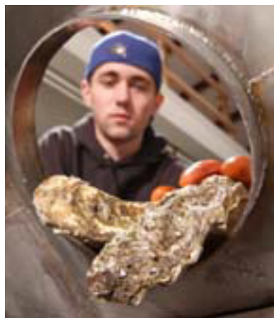
Nisbet worker Brandon Spry puts oysters in a giant canister for high-pressure processing. Photo: Lynn Ketchum
