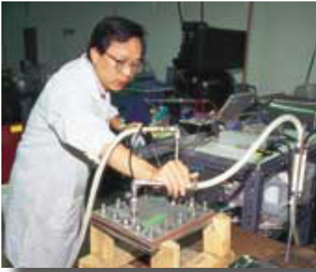
Lihan Huang, an OSU graduate student in food science, works with a membrane filtration system that will recover valuable protein from surimi processing waste water. Photo: Bob Rost
